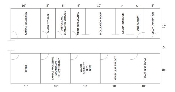
In this design, there is requirement of building with a length of 50 ft and breadth of 25ft. In this design, the entry to each section is separate through the passage. Entry to microbiology section is to media preparation room and exit from observation room. The decontamination room is at the end of the building and so also is the staff rest room. After consultation with an architect and laboratory designer, the layout can be changed without sacrificing the space required for each room.
